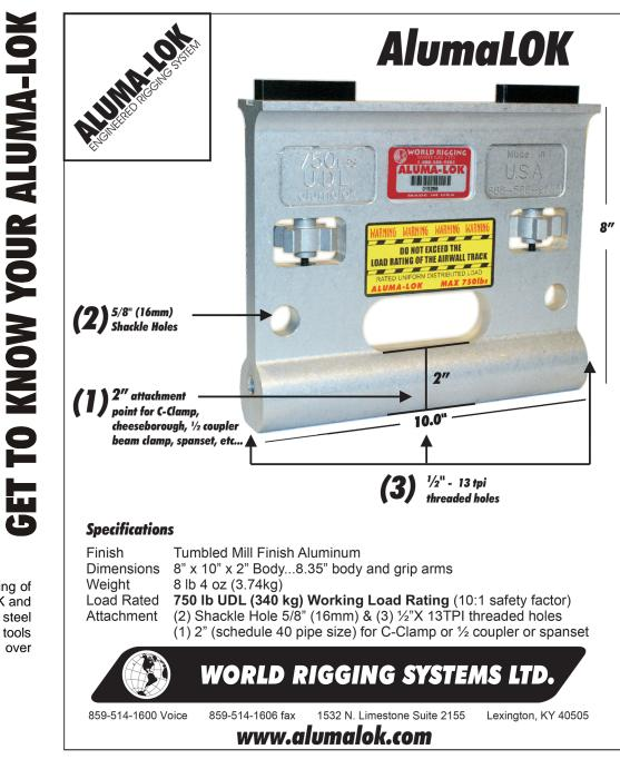
The ALUMA-LOK rigging system has been refined over the years to fit the majority of airwall tracks. There are some tracks out there that the ALUMA-LOK is not compatible with (these oddballs are rare.)
