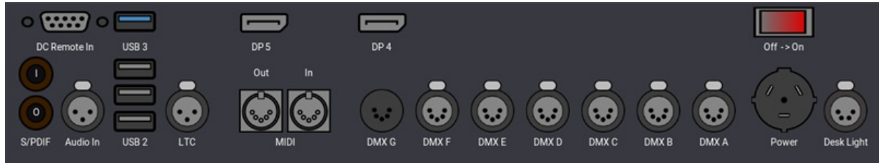
Connector overlay on the right letterbox screen (grandMA3 full-size model)
